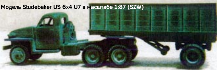
Studebaker US 6x4 tractor & semi-trailer. Unique 2-1/2 - 5 ton classification using 6x4 fifth wheel s. orb. tractor and special trailer. Stock No. MS-48.
